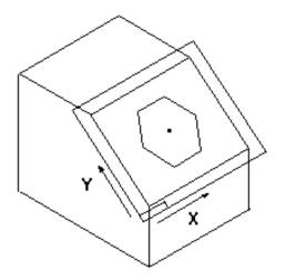
The hexagon is drawn relative to this center point. The system determines whether the profile elements are connected by checking to see if key point relationships exist between the endpoints of the elements.
