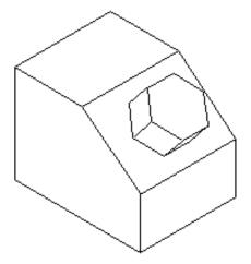
The following program creates the profile and the protrusion feature. The RefPlane variable is assumed to be a public variable that is referencing the reference plane on the face. The size and position of the initial part is known; the center of the face is located at the coordinate (3.5, 2.5, 3.5).
