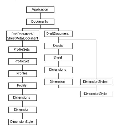
In a Part document, the Dimensions collection is accessed through the Profile object. In the Draft environment, the Dimensions collection is accessed through the Sheet object. The Dimensions collection provides the methods for placing dimensions and for iterating through all the dimensions on the entire sheet or profile.
