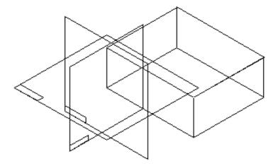
The corner of the block is at the intersection of the three base reference planes. This places the corner of the block at the coordinate (0,0,0), the 6-inch dimension in the positive x direction, the 5-inch dimension in the positive y direction, and the 2-inch dimension in the positive z direction. The cutout to be created is 4 x 1½ inches and ½ inch deep. It is centered on the top face of the block.
