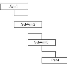
Part4 is a member of SubAsm3, SubAsm3 is a member of SubAsm2, and SubAsm2 is a member of Asm1.
