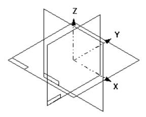
As viewed from a top view, positive x is to the right, positive y is up, and positive z is pointing toward you. The origin of the coordinate system is at the intersection of the three base reference planes as follows:
